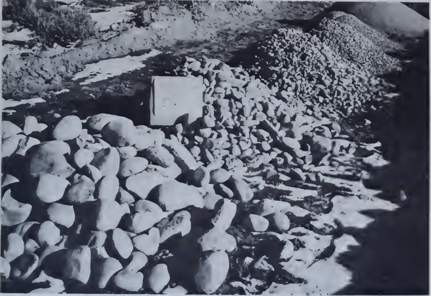
Figure 49.—Graded aggregate piles representing sampled material from trench excavation. P591-421-1217.
